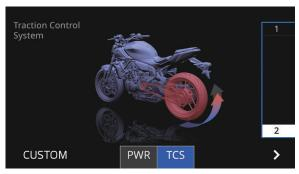
This model uses a variable traction control system. For each setting level, the farther the vehicle is leaned over, the more traction control (system intervention) is applied. There are 2 setting levels available. Level 1 applies the least system intervention, while level 2 applies the most overall traction control to reduce rear wheel slippage.
