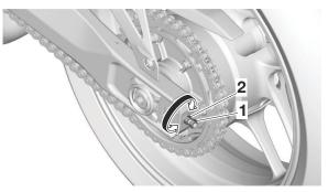
Tighten the wheel axle nut to specification.
