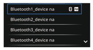
Paired smartphones are listed here. The Yamaha Motorcycle Connect app symbol "[49]" next to a device name indicates that the app is currently connected to the CCU. The Bluetooth symbol "[8]" next to a device name indicates that Garmin Street- Cross is currently connected to the CCU.
