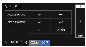
The quick shifter is divided into "QS $\triangle$ " (upshift) and "QS $\bigcirc$ " (downshift) sections. "QS $\triangle$ " and "QS $\bigcirc$ " are not linked and can be set independently.
