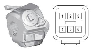
b. Measure the hazard switch resistance.
