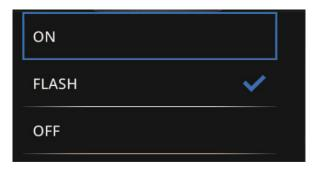
Select "ON" to have the indicator come on at the final r/min. Select "FLASH" to have the indicator start flashing at the initial r/min. When the final r/min is reached, the indicator light will start flashing at a higher frequency. Select "OFF" to turn the indicator off. Short press "
