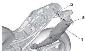
b. Install the rear side cover assembly bolts and quick fastener.
